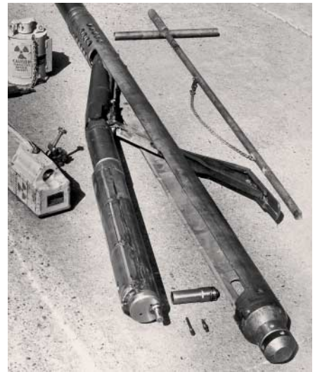
This formation density tool was a major innovation in early nuclear logging technology.
